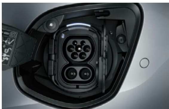
CCS rapid charging port, 80kW max. capacity.
