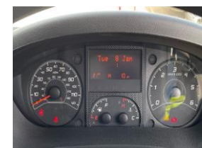
Dials for RPM, fuel and engine temperature - needles have been removed as this information is not required on e-Relay
